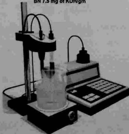
Figure 22.7—Potentiometric titrometer used to determine ANs and BNs.
