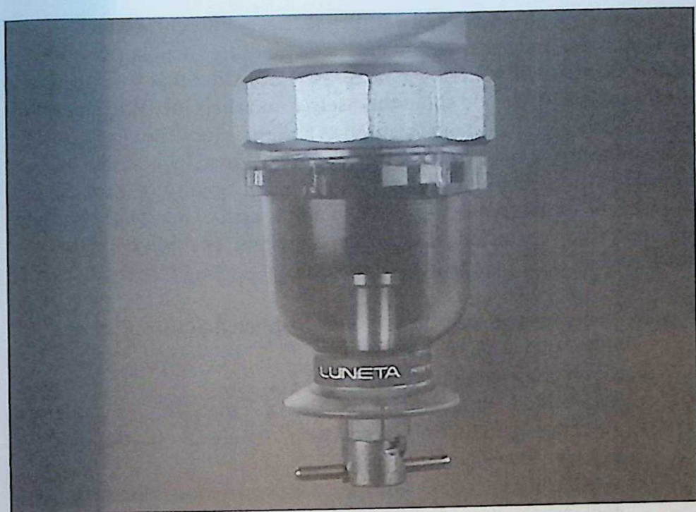
Figure 4.16 Modern bottom sediment and water (BS&W) Bowl Sight Glass.
